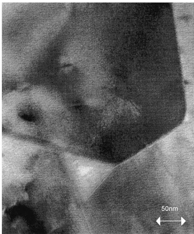
Fig. 6. TEM image of a three-grain junction of sample SF5 with 0.5% \text{SiO}_2 and 0.5% \text{CaO} sintered at 1280 °C.
